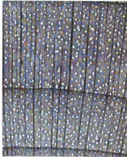
FIG. 330.—Cross-section of Diffuse-Porous Wood. (Hard Maple.) (Bull. 126, U. S. For. Ser.)
